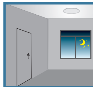
After stand-by period, the sensor switches off the lamp if no motion is detected in its detection zone.
