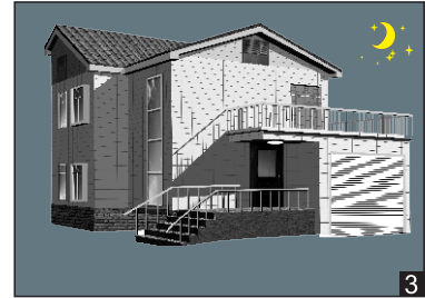
3 After hold time, the lamp gradually dims down if no motion detected.
