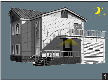
1 No motion detected, the lamp remains at a low light level all the time.
