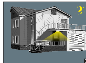
After hold time, the lamp gradually dims to a low light level if no movement detected.
