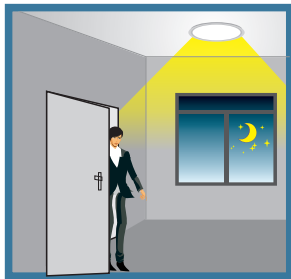
2 With insufficient ambient light, the sensor switches on the lamp when motion is detected.
