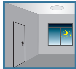
4 After stand-by period, the sensor switches off the lamp if no motion is detected in its detection zone.
