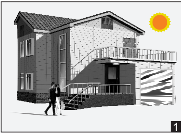
1 With sufficient ambient light, the sensor does not switch on the lamp.
