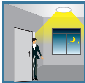
With insufficient ambient light, the sensor switches on the lamp when motion is detected.
