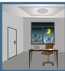
If with insufficient ambient light, the lamp dims to a stand-by dimming level (Set in the motion sensor) when no motion detected during hold time, and then switches off after stand-by period.
