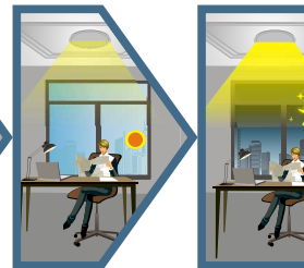
The lamp lights on 100% illumination or dims to maintain the preset illumination level against ambient light.
